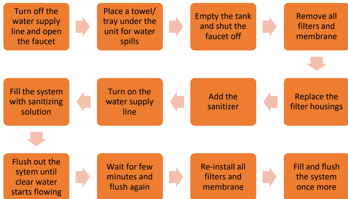
Fig 5.2.7: Steps to sanitize an RO system
