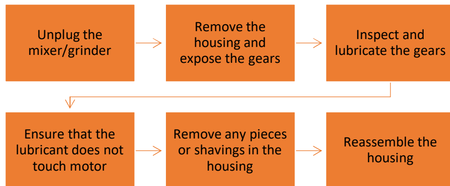
Fig 6.2.2: Servicing the gears
